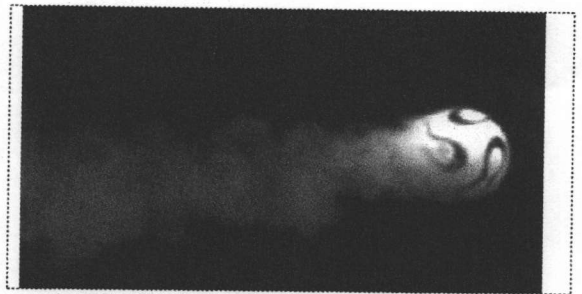
Fig. 1 Flow visualization of vortex behind the real flight soccer ball. Flow is from right to left.
